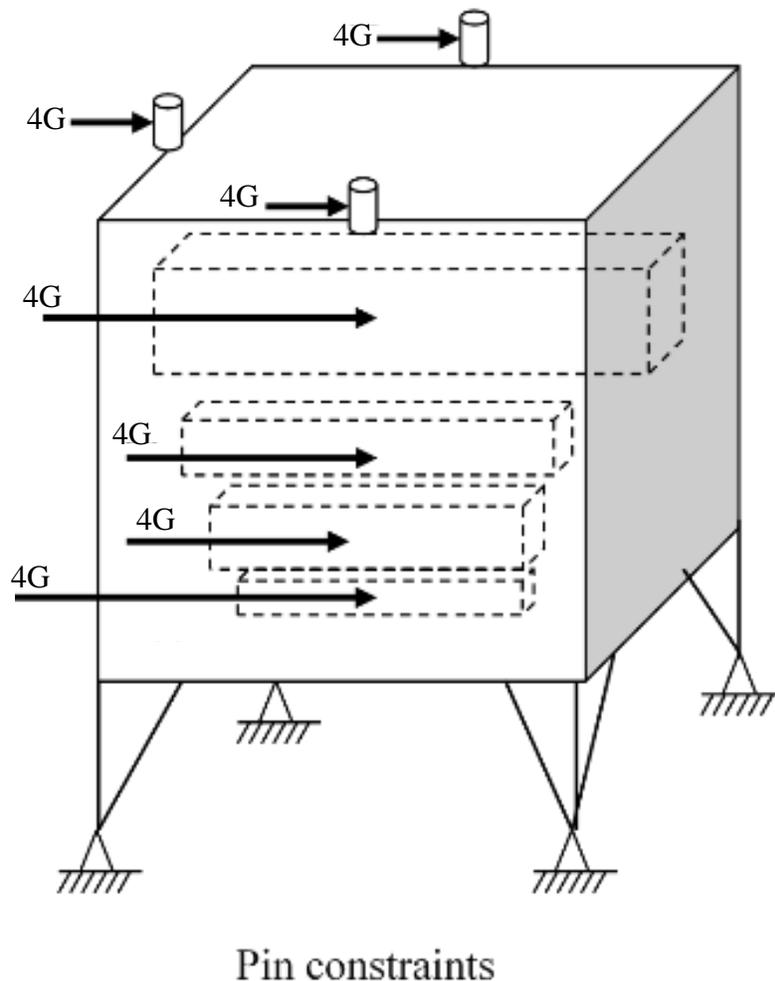
**Figure 5: Load Case #4 – Gondola Lateral Loading**
