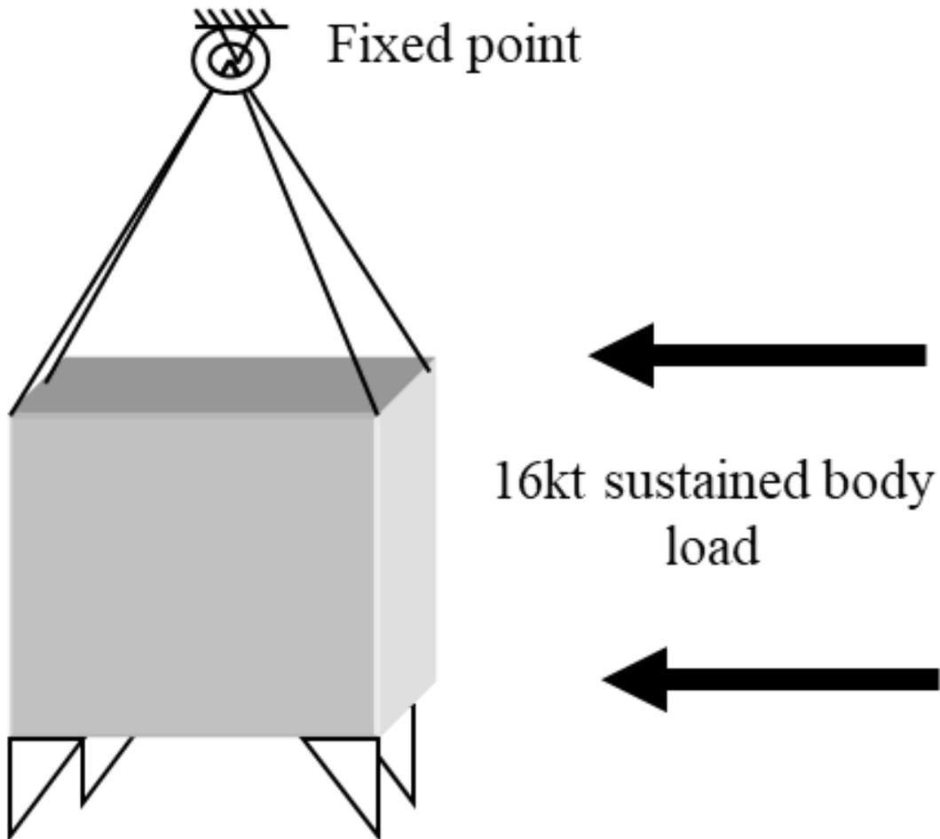
**Figure 6: Load Case #6 – Sustained Wind Loading**
