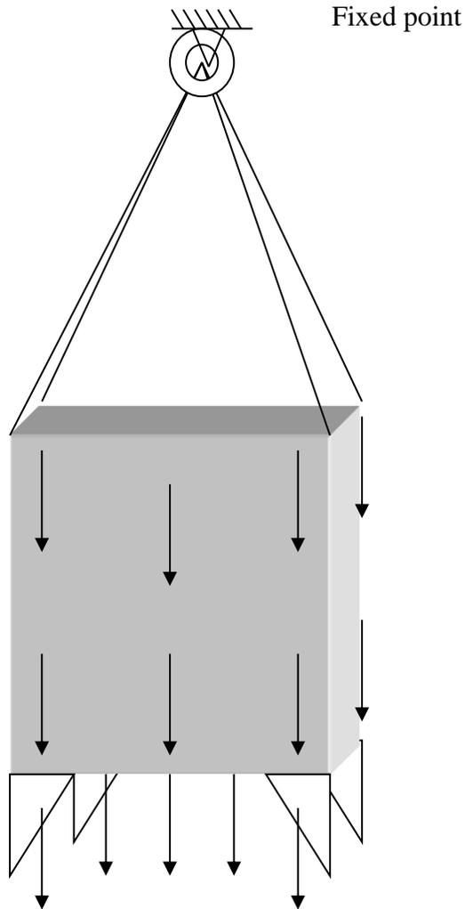
**Figure 2: Load Case #1 – Gondola Vertical Loading**
