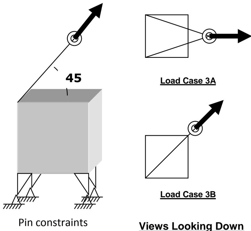
**Figure 4: Load Case #3 – Off-Vertical Gondola Loading**
